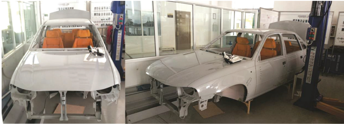
Figure 8. The model for using the gap and flushness as calibration artefact
