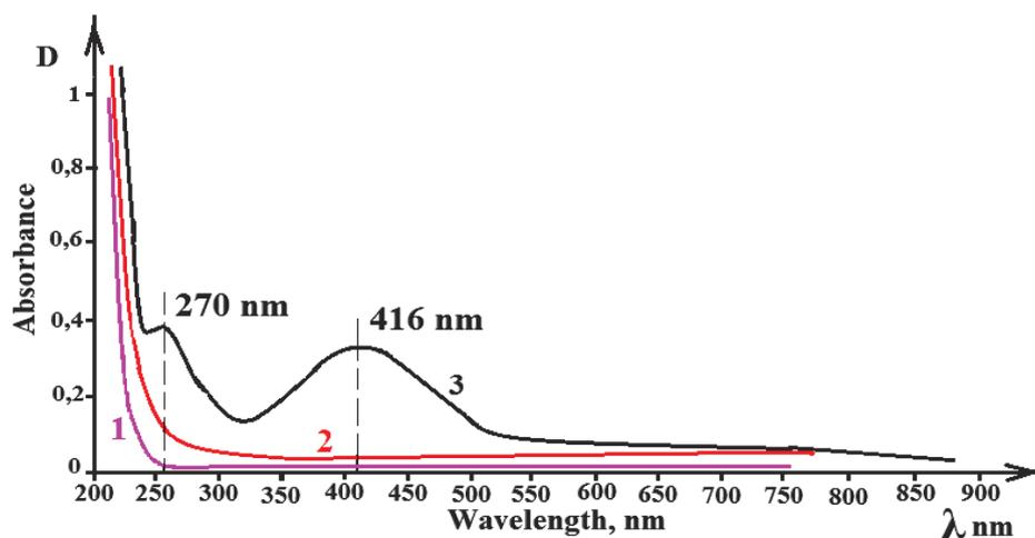
The UV-irradiation duration for the samples was equal to 25 minutes,  $[\text{Na-CMC}] = 8 \times 10^{-3} \text{ mol/L}$  (2 wt. %);  $[\text{AgNO}_3] = 3 \cdot 10^{-5} \text{ mol/L}$  (0.25 wt. %).
