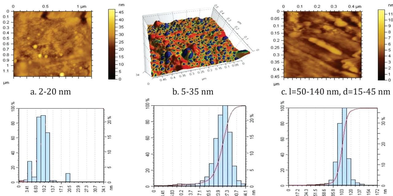
Concentration of  $[Na-CMC] = 8 \times 10^{-3} \text{ mol/L}$ ; UV-irradiation time is 30 min.
