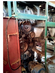
7-rasm. UXK paxta tozalash mashinasining 1-tozalash zonasini uchun kinematik sxemasi va tasmalarni o'rnatish jarayoni
